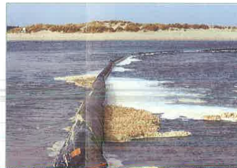
Right: Inflatable oil booms are often used to surround and contain oil and prevent it from reaching the shore.
