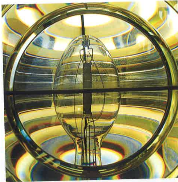
Lighthouse Lens. Cut glass in a Fresnel lens focuses light into a bright beam.
